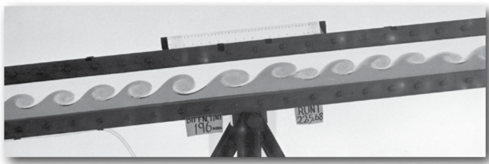
Figure 3.8: Tilting tank laboratory experiment in which a dense (here, dark) layer of fluid underlies a lighter fluid initially at rest. When the tank is tilted, buoyant forces accelerate the denser fluid down and the lighter fluid up the slope, thereby creating a velocity gradient across the interface and subsequent billow formation. From: Thorpe, S.A. 1971. Experiments on the instability of stratified shear flows: Miscible fluids. Journal of Fluid Mechanics 46: 299 - 319.
